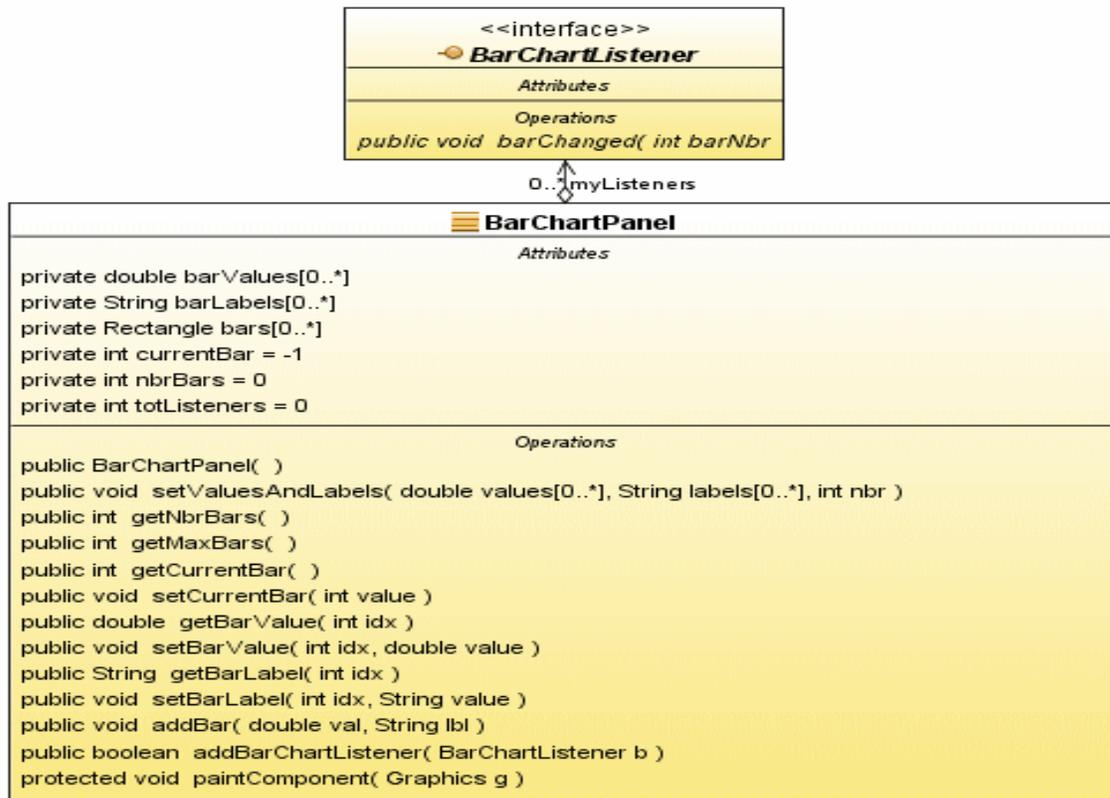
Figure 3: UML diagram for a typical BarChartPanel implementation.
