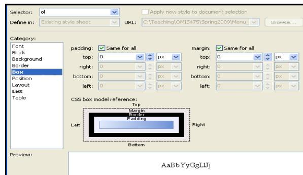
**Figure 3. Reset the Padding & Margins in CSS**
